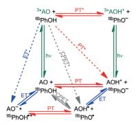
Figure 2: PCET mechanistic pathways between photo-excited acridine orange (AO) and tri-tert-butylphenol (<sup>ttb</sup>PhOH).
