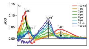
Figure 3: Photo-induced transient absorption spectra of 40  $\mu$ M acridine orange during the PCET mechanism with 1 mM tri-tert-butylphenol ("bPhOH) in acetonitrile; excitation was at 425 nm.
