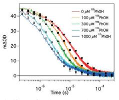
Figure 4: Triplet lifetime of acridine orange in the presence of increased concentrations of tri-tert-butylphenol (<sup>ttb</sup>PhOH) in acetonitrile; lifetimes were recorded at 560 nm.
