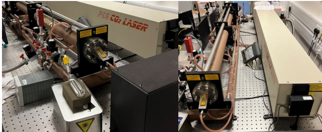
Figure 1. Optical images from the experimental setup used by the University of Glasgow researchers showing an Edinburgh Instruments FIR-295 gas laser, optically pumped by the PL5 CO 2 laser. Images courtesy of University of Glasgow.
