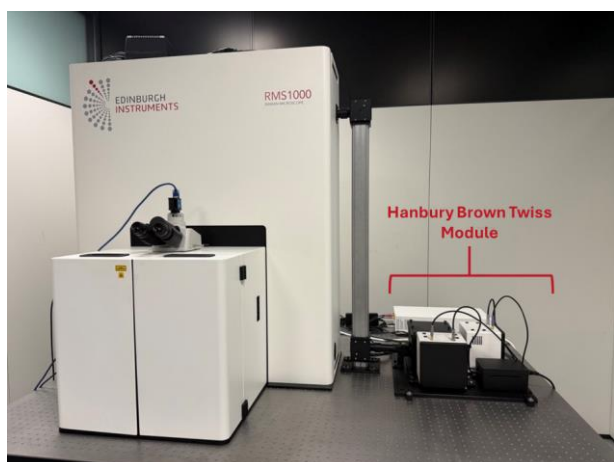
Figure 1. RMS1000 configuration for g^{(2)} correlation measurements showing coupling to antibunching HBT module.
