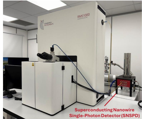
Figure 4. RMS1000 coupled to SNSPD for NIR antibunching experiments.
